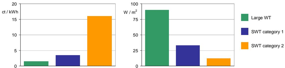
Figure 3: Operational costs (left) and specific power output (right) for large WT and SWT in the WMEP
