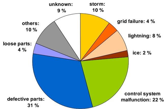
Figure 4: Frequency of causes for failure for all SWT (both categories) in the WMEP
