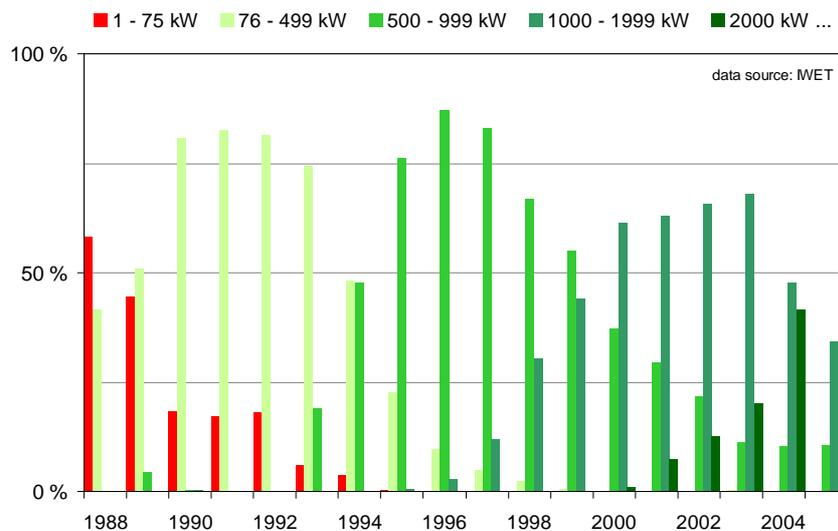
Figure 2: Share of newly installed wind turbines in Germany per power class
