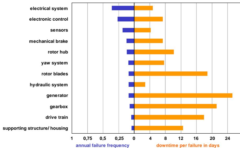
Figure 6: Frequency of failure of main components and related downtime for all SWT (both categories) in the WMEP
