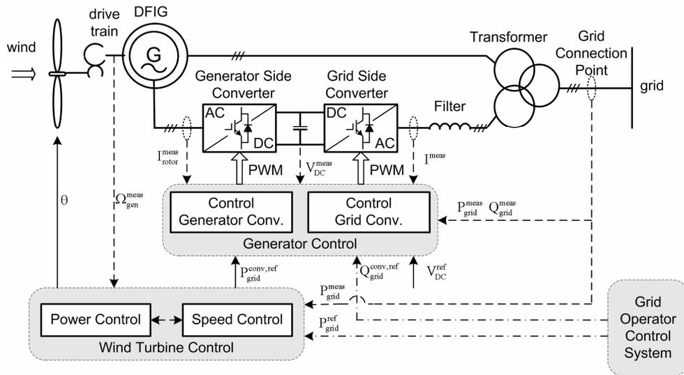
Fig. 10. Control of wind turbine with doubly-fed induction generator system [35].
