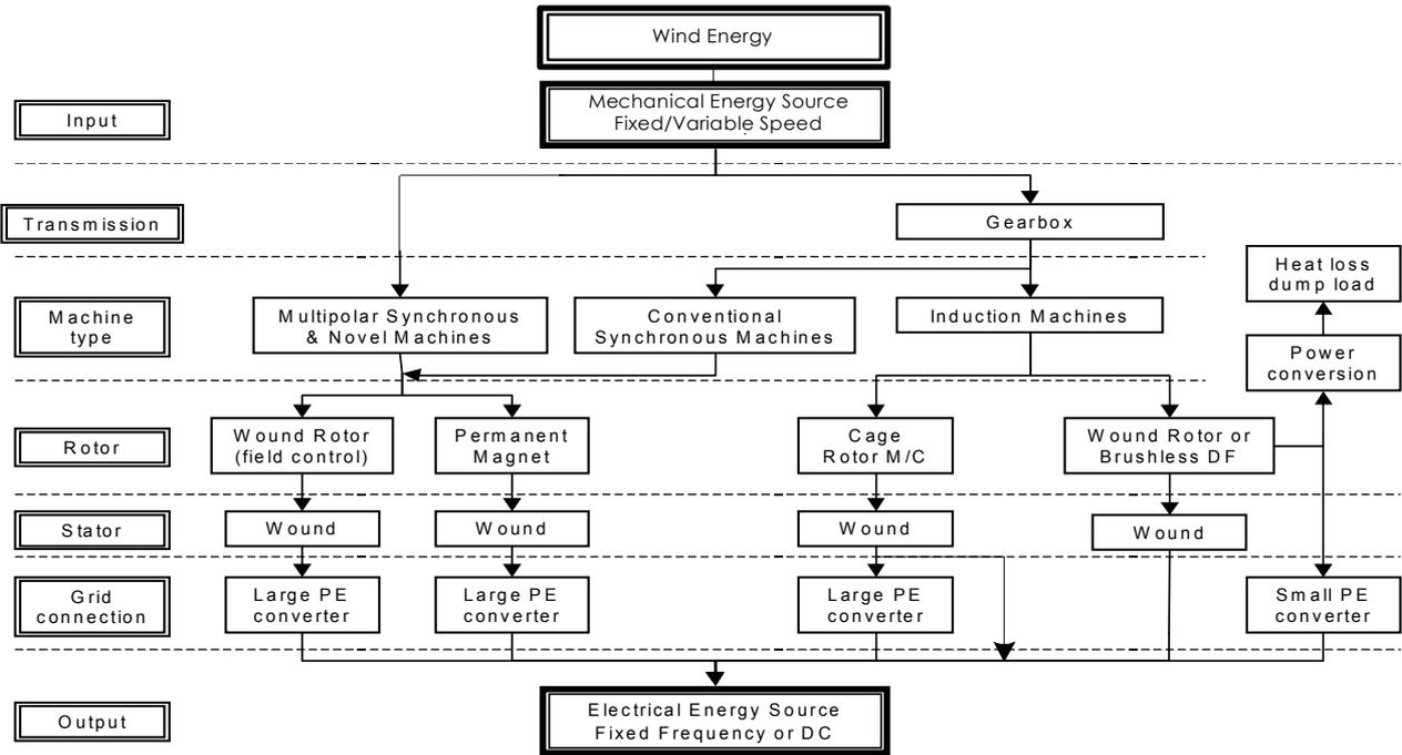
Fig. 5. Road-map for wind energy conversion. PE: Power Electronics. DF: Doubly-fed [15], [22].
