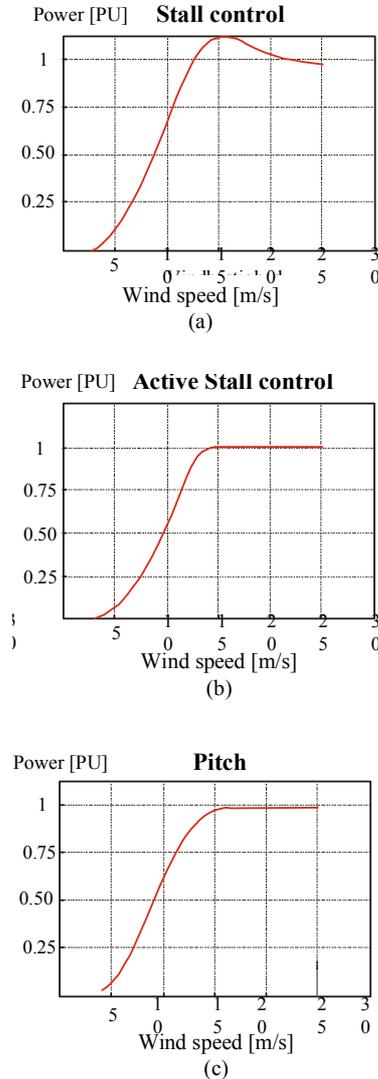
Fig. 7. Power characteristics of fixed speed wind turbines.
