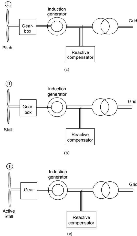
Fig. 6. Wind turbine systems without power converter but with aerodynamic power control.
