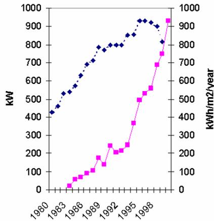
Fig. 14. Average size of wind turbines and produced energy pr. m2 swept area pr. year in Denmark.
