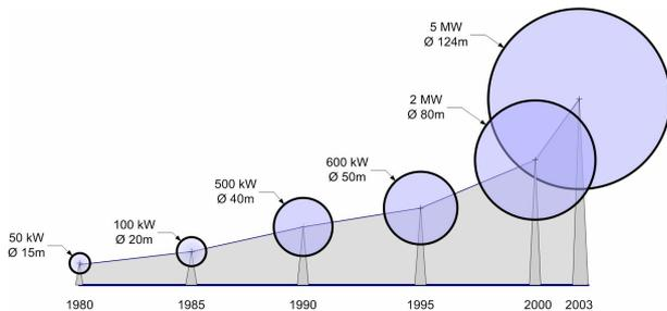
Fig. 16. Development of wind turbines during the last 25 years.
