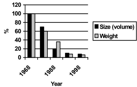
Fig. 2. Development of a 4 kW standard industrially adjustable speed drive during the last 25 years [5].
