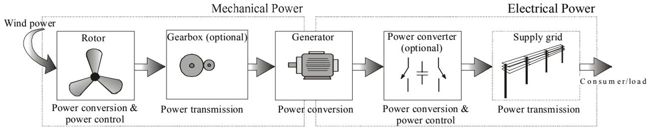
Fig. 4. Converting wind power to electrical power in a wind turbine [17].
