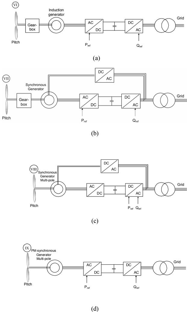
Fig. 9. Wind turbine systems with full-scale power converters.
