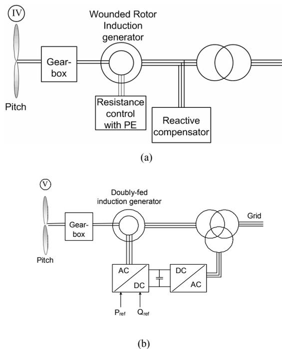
Fig. 8. Wind turbine topologies with partially rated power electronics and limited speed range.
