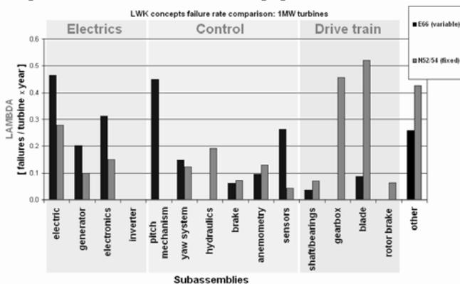
Figure 4 : Comparison between failure rates of the Group 2, larger, WT Concepts
