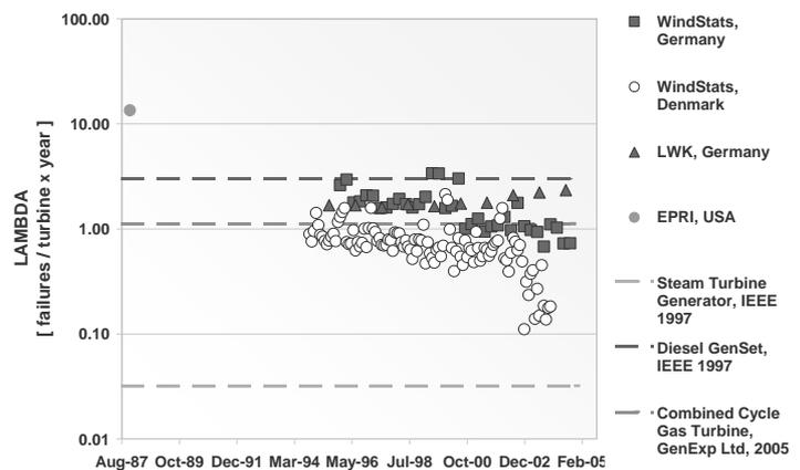
Figure 1: The failure rates of Onshore Wind Turbines taken from WindStats [4] and compared with other power sources.
